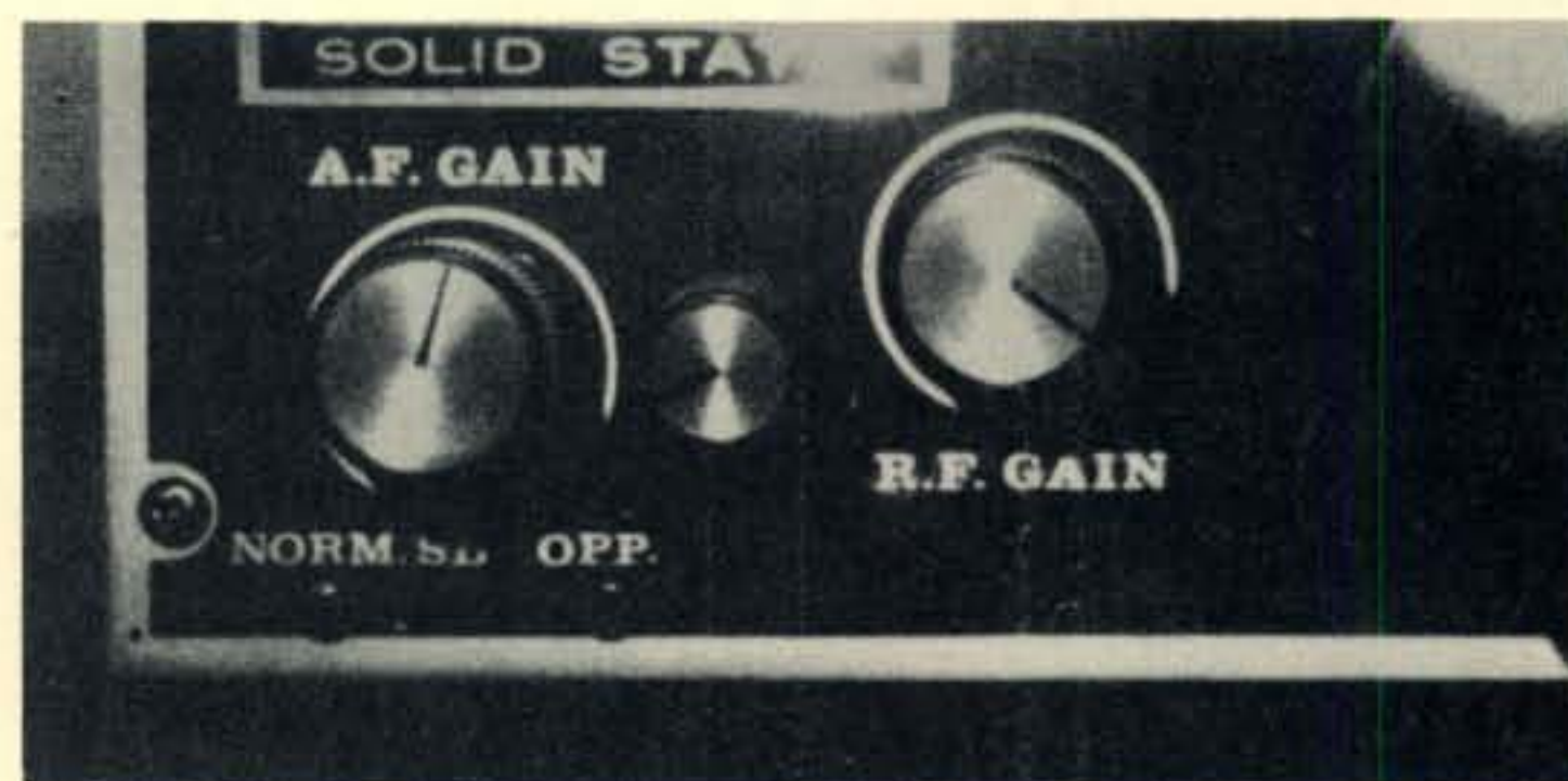
The s.w.r. Sensitivity control knob is located between the a.f. and r.f. gain controls at the lower left side of the Atlas front panel. The panel light dimmer switch is used for meter switching, while the panel lights are permanently wired for the desired brilliance.
