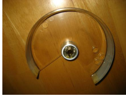
View of repaired hub that has stress cracks
